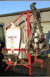
A superbly engineered range of tractor mounted sprayers using the latest technology and materials to produce a well equipped sprayer with booms up to 15 metres and tank sizes up to 1500 litres.
