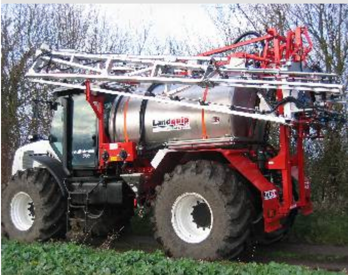
Multidrive equipped with 24m LR Alu-light boom and 4000 litre stainless cylindrical tank
