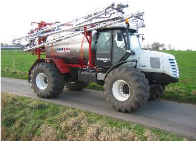
Multidrive equipped with 24m LR Alu-light boom and 4000 litre stainless cylindrical tank
