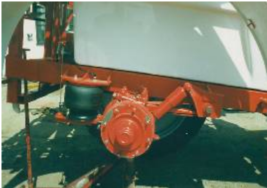
Pneumatic level ride load sensing air suspension axle (optional extra)
