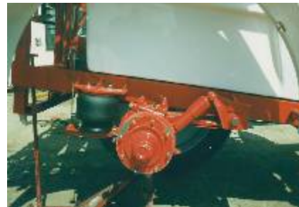
Pneumatic level ride load sensing air suspension axle
