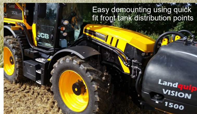
Fastrac 4220 equipped with 24 metre bi-fold aluminium boom + Vision 1500 front tank = total capacity 4000 litres (4400 litres with Vision 1900)
