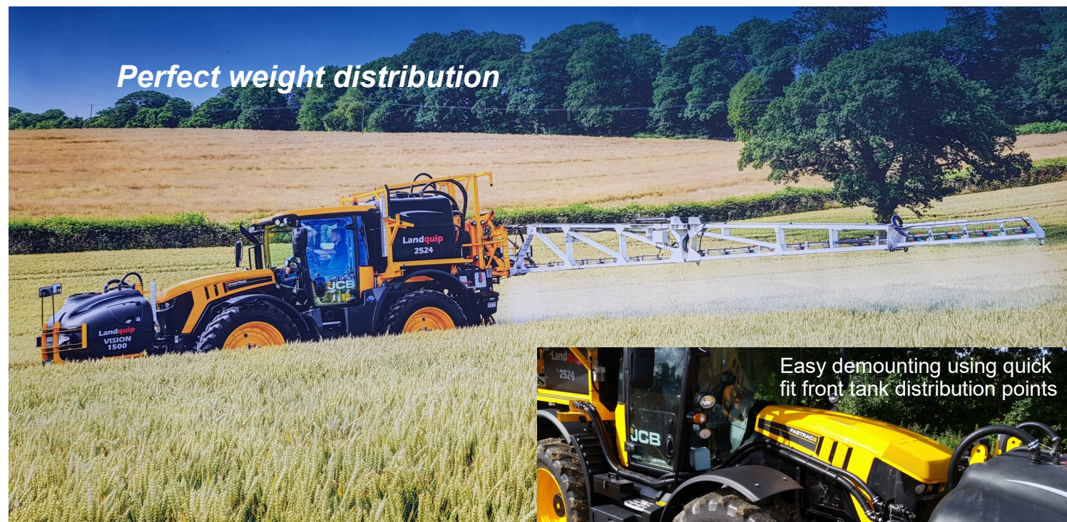
Fastrac 4220 equipped with 24 metre bi-fold aluminium boom + Vision 1500 front tank = total capacity 4000 litres (4400 litres with Vision 1900)
