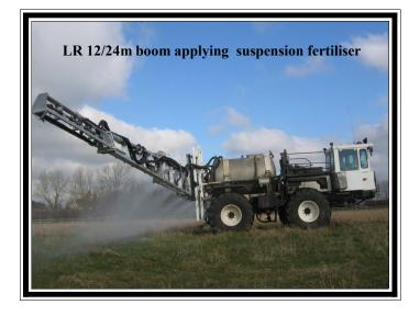
The Alu-light range of aluminium booms from 24 to 48 metres can be fitted to most makes of sprayer
